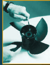
4. Tighten bolts w/ allen wrench.
