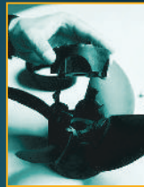
2. Separate the propeller to release blades. Change blades & reassemble unit.
