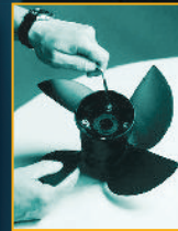
3. Tighten bolts w/ allen wrench.
