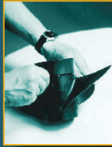
3. Grasp two opposite blades and turn to the right pitch on the scale.
